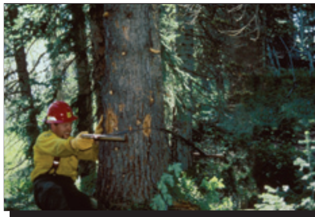
Figure 5-29—Gunning the saw helps determine the specific direction of the undercut. (Photo has been digitally altered to remove distracting items.)
