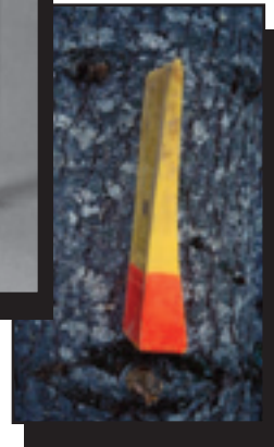
Figure 5-14—Triple-taper wedges allow a short wedge to provide as much lift as a longer wedge but require more force to drive.
